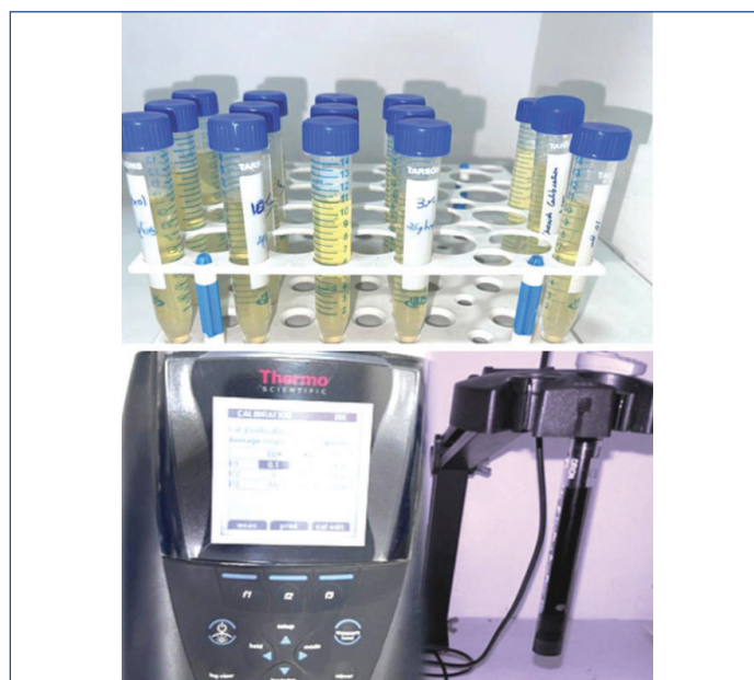
[Table/Fig-2]: Assessment of fluoride release using ion selective electrode analyser.
